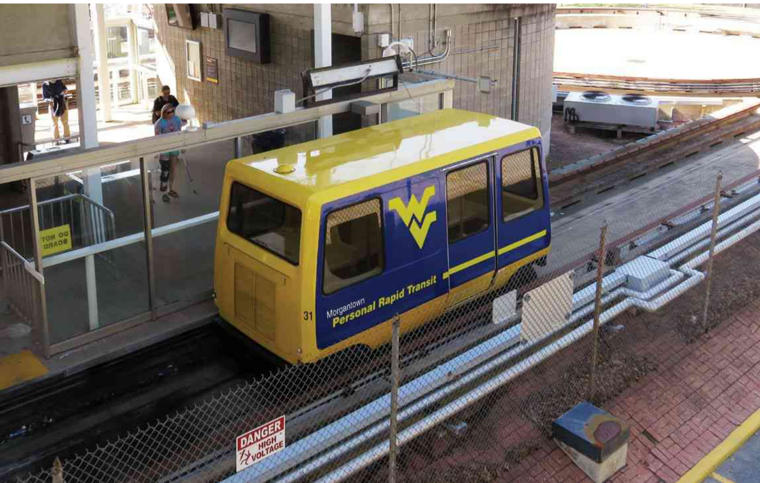
▼ Morgantown, USA America's one and only personal rapid transit (PRT) system connects the three Morgantown campuses of West Virginia University and the city's downtown area. The driverless system was a government-funded experiment which opened in 1975. Like all PRT systems, stations are built on sidings, which allows vehicles to bypass stations and enables express trips between any two station pairs. Photo: Jae69376 (above), Antony-22 (below)
