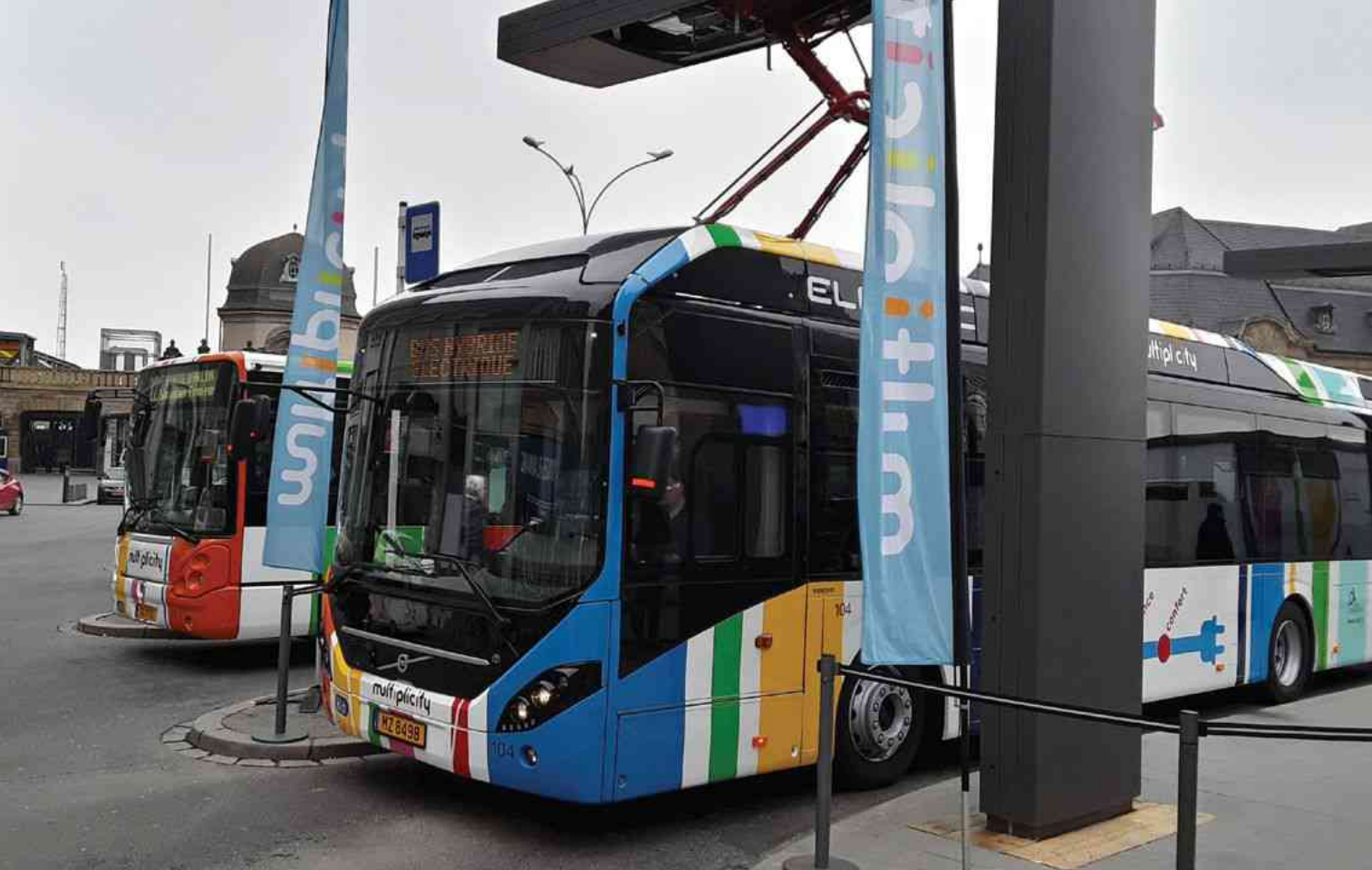
▲ Luxemburg Volvo 79 Electric Hybrid from AVL (Ville de Luxembourg) at a fast charging station at Central Station in Luxembourg. Photo: GilPe
