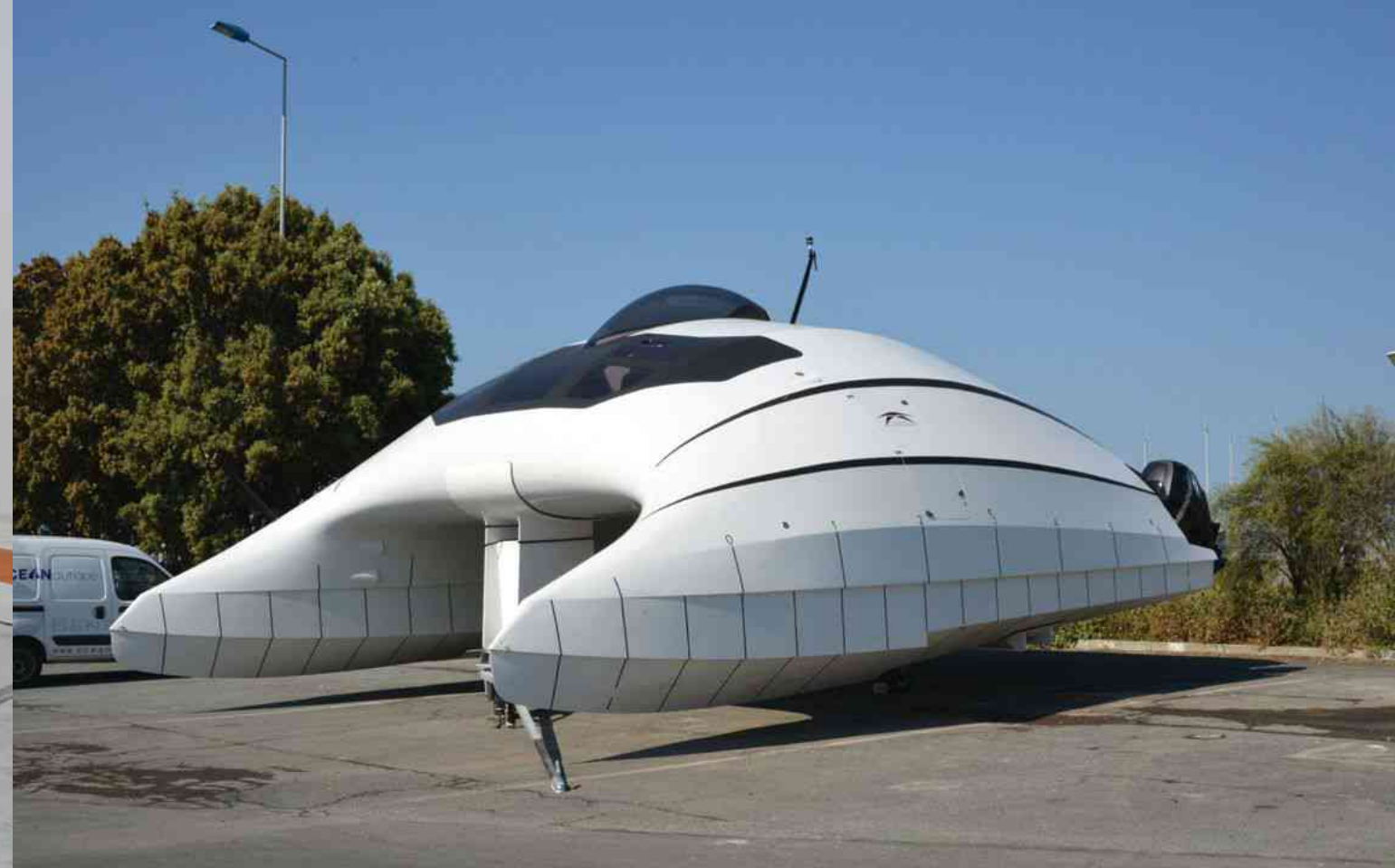
▲ France The "Lili" prototype from Advanced Aerodynamic Vessels make the most of aerodynamics and rely on the air to lighten the weight of the boat and thus go faster (up to 60 knots or over 110 km/h) whilst using less fuel. Photo: Jean-Pierre Bazard.
