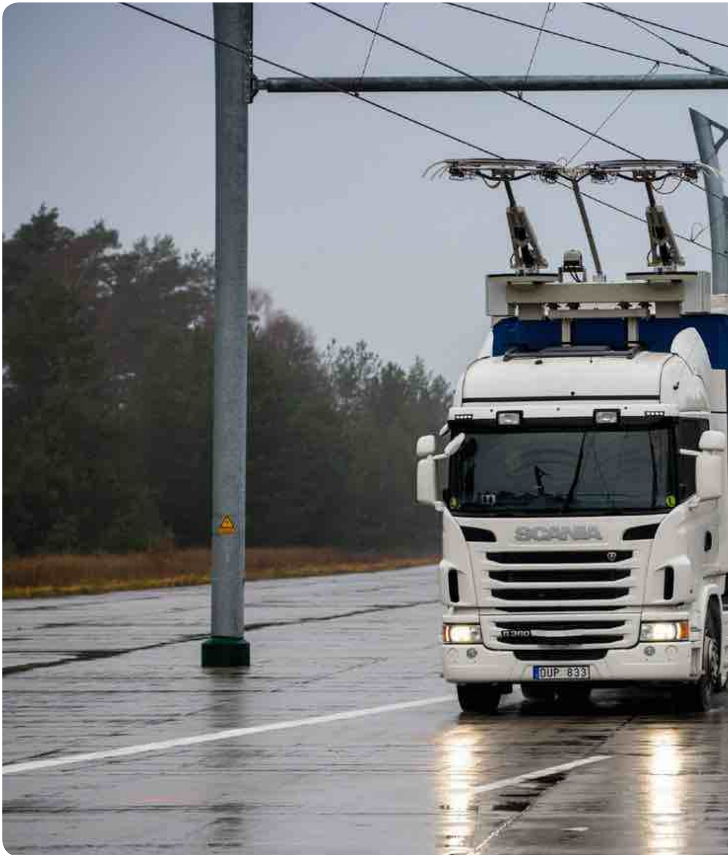
The first eHighway system on a public road opened in June 2016. For the coming two years, a Siemens catenary system for trucks will be tested on a highway north of Stockholm. Source: Scania / CV AB
