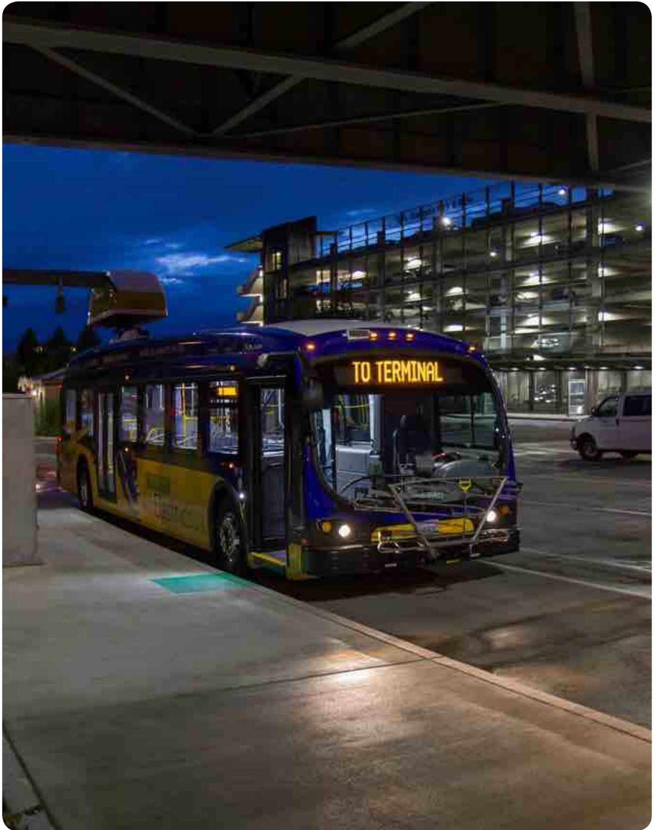
KCM 4602 (Proterra) charging at the layover area at Eastgate Transit Center, King County. The fast-charge option can be fully charged in ten minutes, while the extended range option can be fully charged in approximately one hour. Source: Atomic Taco
