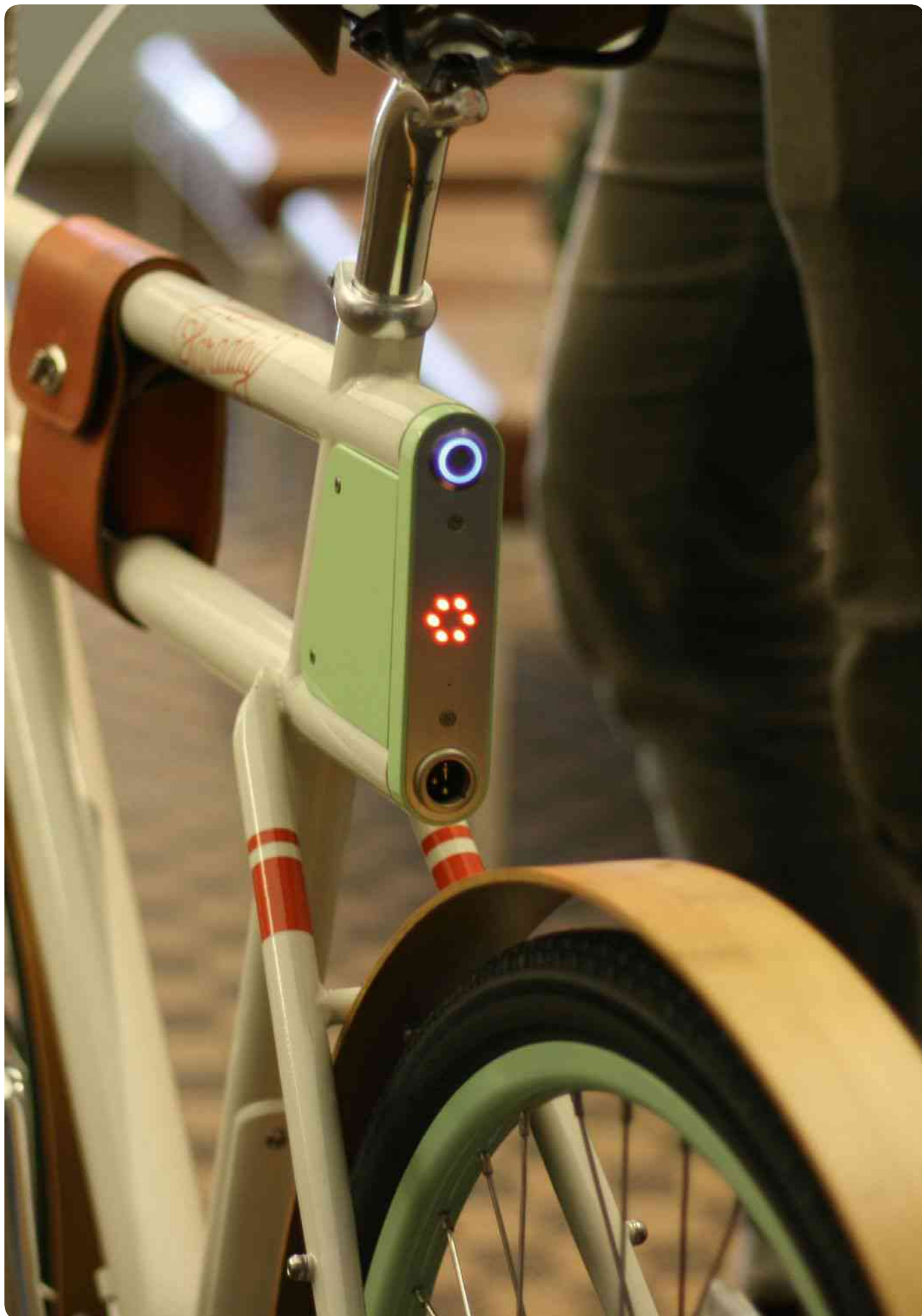
The Faraday Electric Bike has a simple classy design with batteries in the downtube and a front hub motor. Source: Richard Masoner
