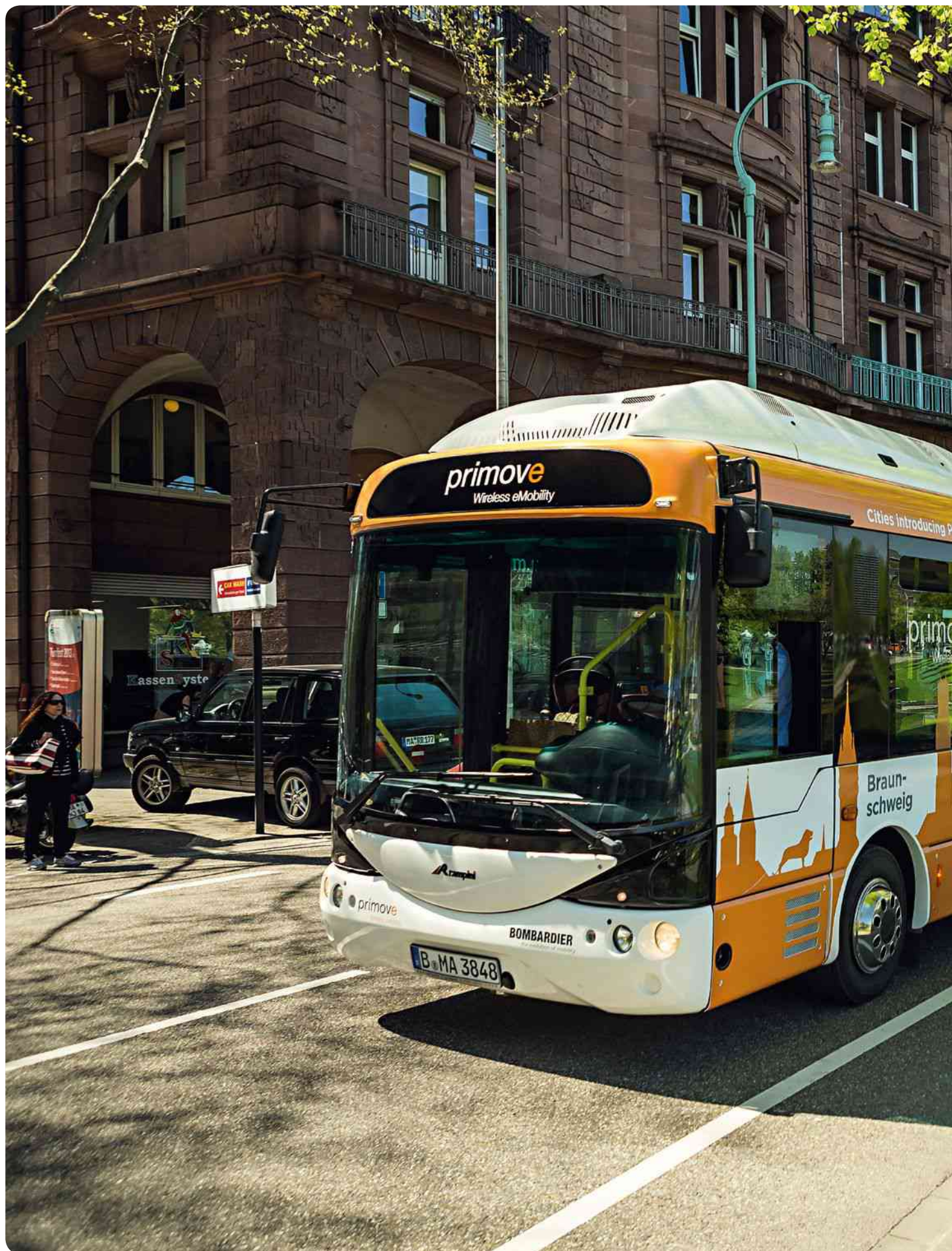
BOMBARDIER PRIMOVE: a wireless and contactless charging system for clean, quiet and convenient e-buses in the historic city centre of Bruges, Belgium. Source: Bombardier
