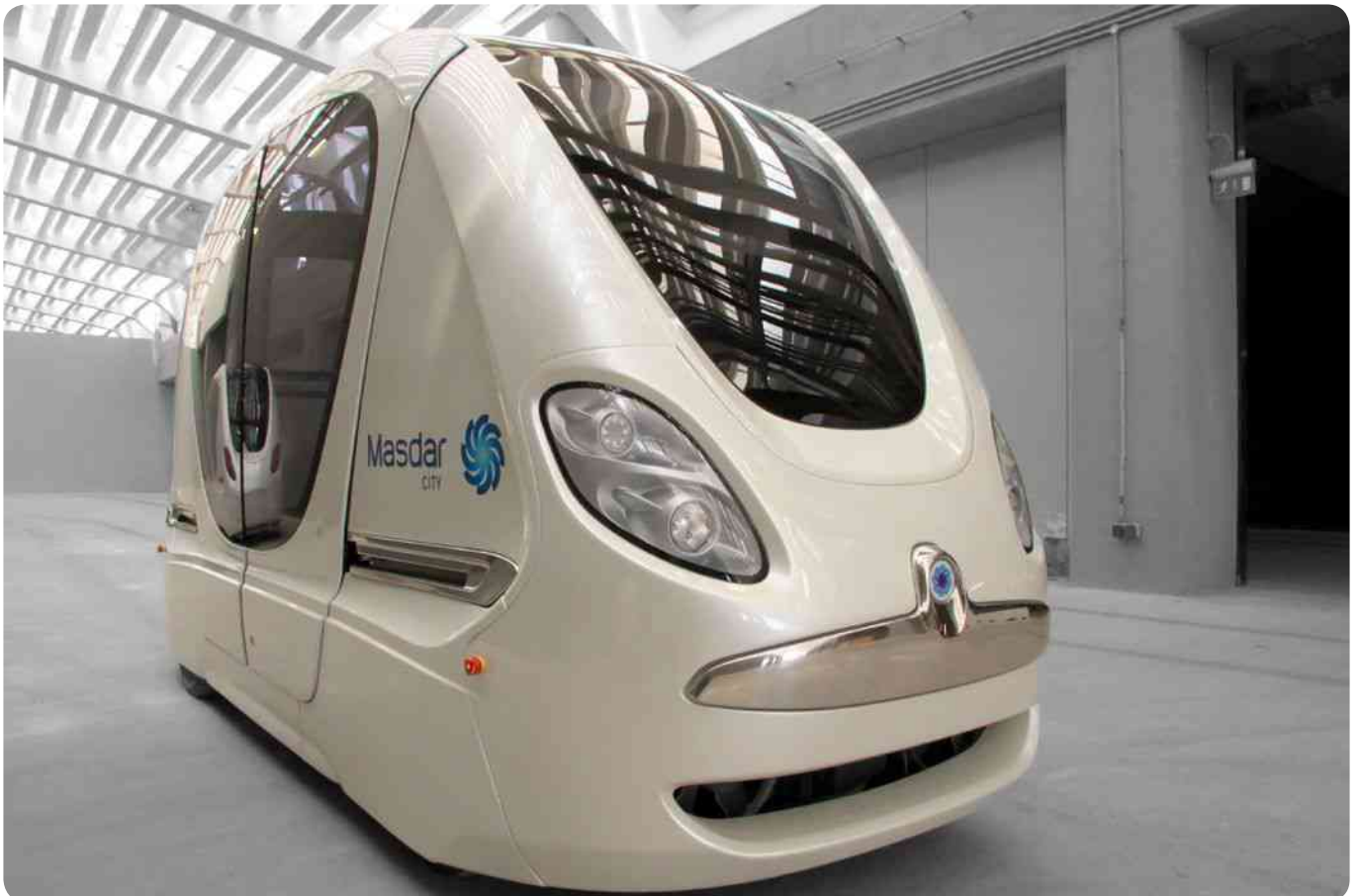
The Personal Rapid Transit (PRT) – also known as podcars – is an automated guideway transit (AGT) system that operate digitally on specifically designed magnetic paths. Since 2010, a 10-unit PRT system has been operating in Masdar City, UAE. Source: 2getthere
