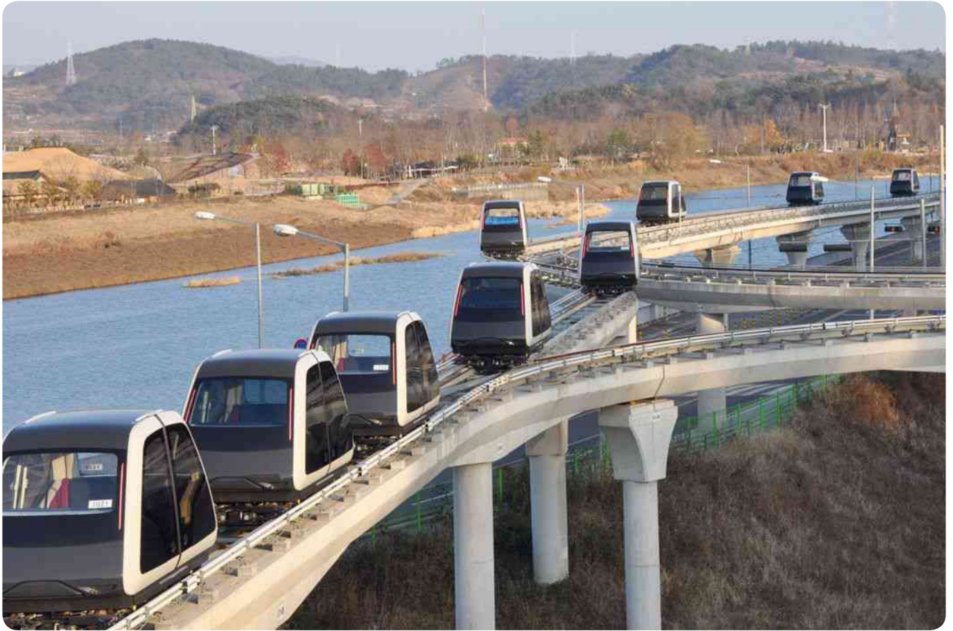
Personal Rapid Transits (PRT) move irregular flows of people, going in different directions, and allows point-to-point travel, bypassing intermediate stations. Source: Vectus
