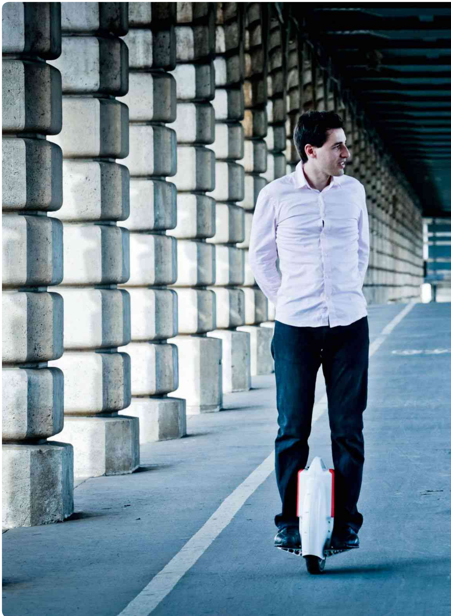
Urban mobility is mainly about travelling short distances, done by different modes. On the market in France and Belgium since 2015, these self-balancing unicycles are powered electrically. This new 10 kg compact vehicle is easy to carry and can cover up to 10 km at about 10-15 km/h. Source: Solowheel
